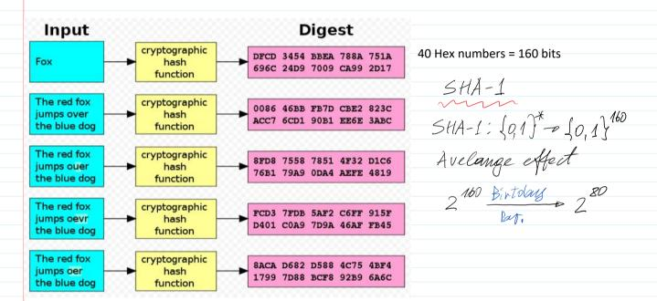
A cryptographic hash function (specifically <u>SHA-1</u>) at work. A small change in the input (in the word "over") drastically changes the output (digest). This is the so-called avalanche effect.
